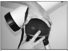
Figure 2-9 – Removing the Battery Compartment Lid
