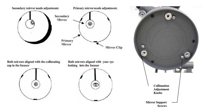
Adjustments to the collimation of the telescope can be made by turning the collimation adjustment knobs located at the rear of the optical tube. First loosen the three Phillips head screws on the rear cell of the tube. Turn each collimation knobs, one at a time, until the reflected image of your eye in the secondary mirror is centered in the primary mirror. Once the telescope is collimated, tighten the Phillips head screws until you feel a slight resistance. Do not over tighten the screw.
